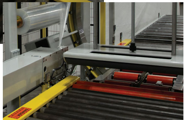
RIGHT: Hold-down platen ensures the load remains stable during wrapping
