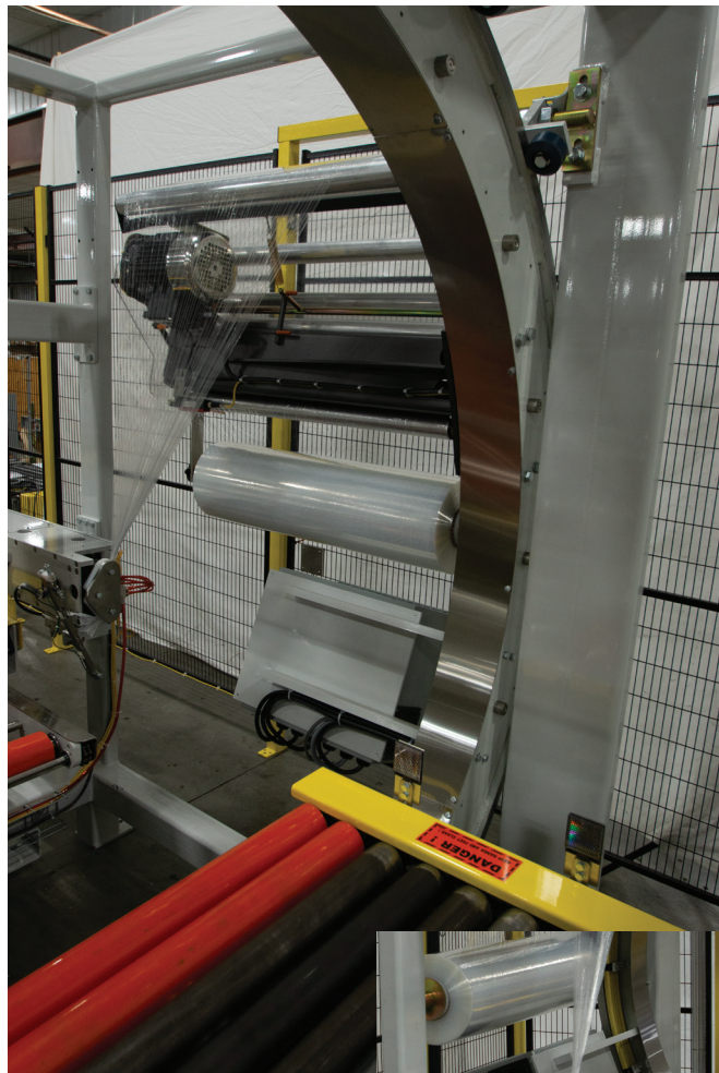
TOP: Film shown threaded and ready to wrap
