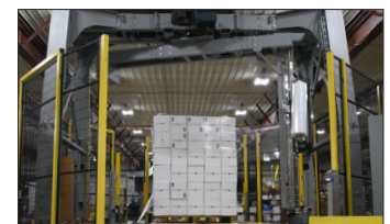
Ultra-Stable "A" Frame Design Heavy-duty steel tube structure minimize machine wear and tear for long product life. Stable frame ensures reliable and consistent performance, maximizing uptime, minimizing operational costs.
