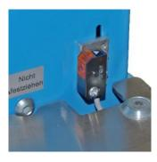
The photocell is height-adjustable and is used to automatically trigger the banding process.
